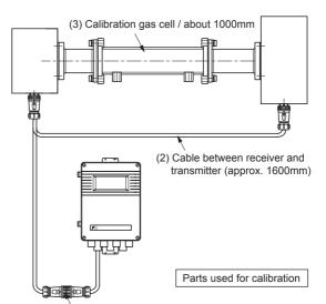
(1) Cable between receiver unit and control unit
