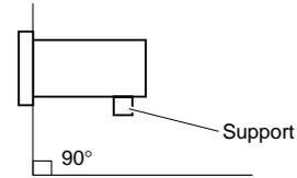
**Note:** Instrument mass of more than 70% should be supported at the bottom of the case.
